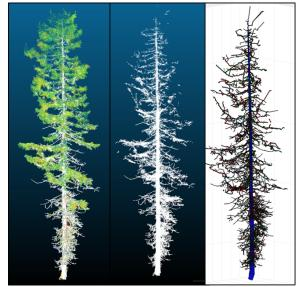
Figure 1 (left to right): TLS clipped 3D scan, scan with leaves removed, QSM model from point cloud
