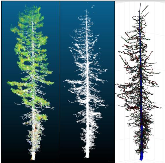
Figure 1 (left to right): TLS clipped 3D scan, scan with leaves removed, QSM model from point cloud
